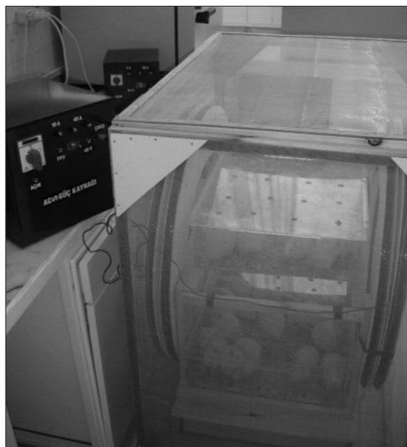
Figure 1. MF exposure in Faraday and flexiglass cages.
