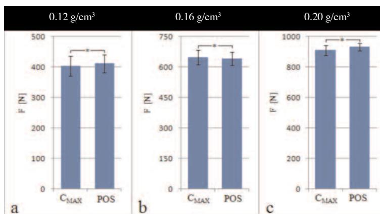
**Figure 5.** In the 0.12  $g/cm^3$  specimen, the mean  $C_{MAX}$  is 403.65 N and the mean POS is 411.51 N (a). In the 0.16  $g/cm^3$  specimen, the mean  $C_{MAX}$  is 648.97 N and the mean POS is 641.82 N (b). In the 0.20  $g/cm^3$  specimen, the mean  $C_{MAX}$  is 910.92 N and the mean POS is 932.68 N (c). \*Not significantly different ( $p > 0.05$ ).  $C_{MAX}$ , maximum compressive force; POS, pullout strength.
