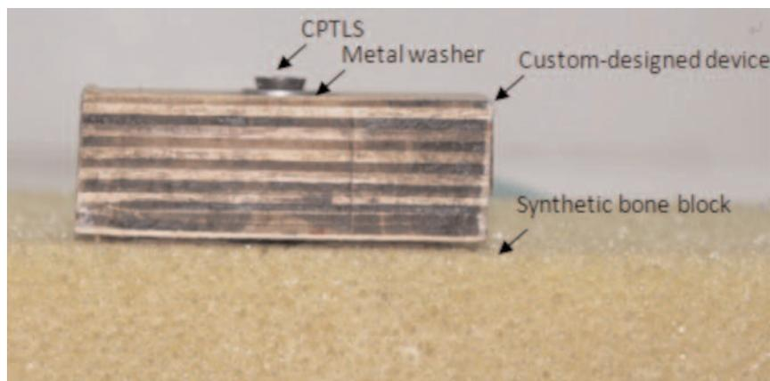
**Figure 3.** The system for measuring  $C_{MAX}$  consists of the CPTLS, a metal washer, the custom-designed device, and the synthetic bone block.  $C_{MAX}$ , maximum compressive force; CPTLS, combined partially threaded cancellous lag screw.
