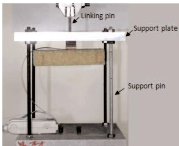
**Figure 4.** The system for measuring POS consists of a linking pin, a screw extraction grip, two aluminum support plate and four support pins. After the screw had been inserted without producing any compression, it was pulled out using this system and BOSE3510-AT testing machine. POS, pullout strength.
