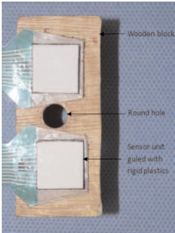
**Figure 2.** The custom-designed device, consisting of a wooden block with a 7-mm round hole in the middle and two sensors glued with rigid plastic, for measuring  $C_{MAX}$ .  $C_{MAX}$ , maximum compressive force.
