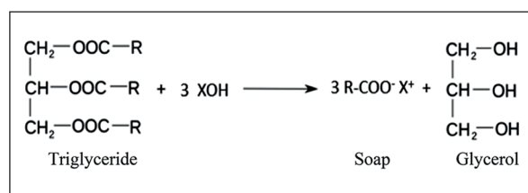
Figure 1. Saponification reaction. Where X = Na or K and R is a hydrocarbon chain of 10 to 18 carbon atoms.
