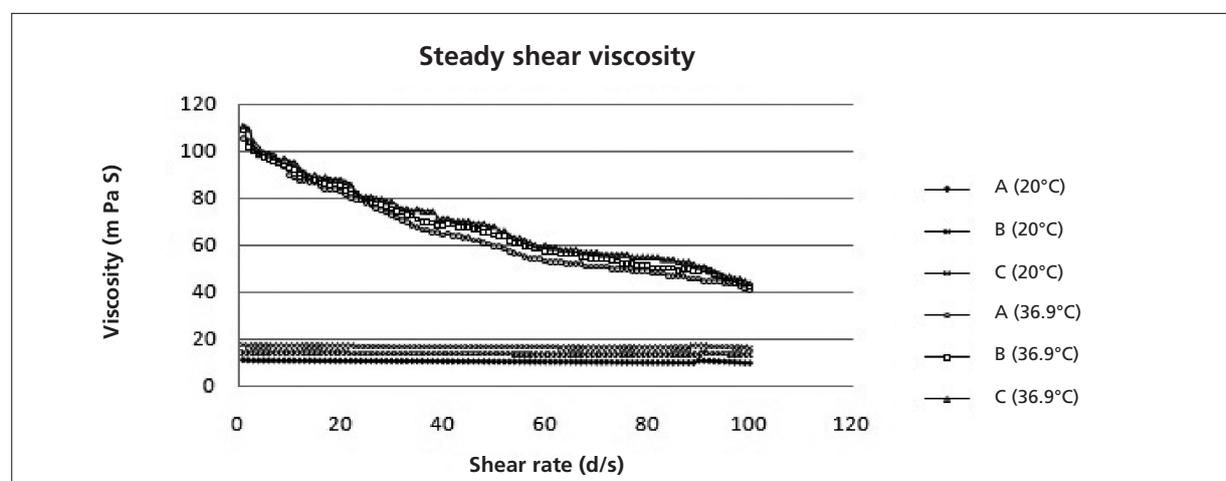
Figure 1. Viscosity vs shear rate graph at 36.9°C and 20°C.
