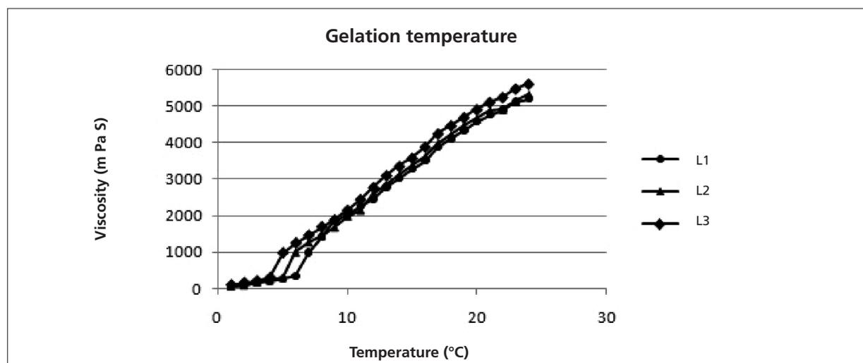
**Figure 2.** Viscosity vs temperature graph showing gelation temperature.
