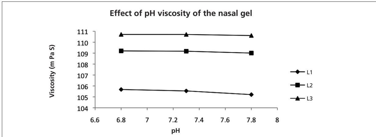
Figure 3. Viscosity vs pH graph at 60 s<sup>-1</sup>shear rate.
