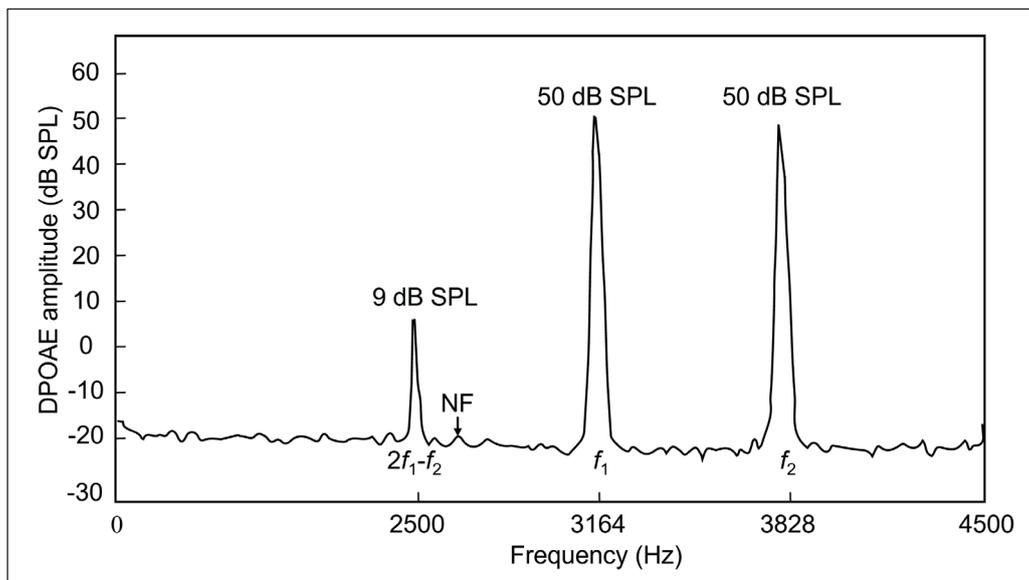
**Figure 2.** The DPOAE spectrums of normal-hearing people. The frequencies of the two initial pure tones are  $f_1 = 3164$  Hz,  $f_2 = 3828$  Hz. The intensities are  $L_1 = L_2 = 50$  dB. The frequency of DPOAE is  $2f_1 - f_2$  which is 2500 Hz. DPOAE: distortion product otoacoustic emission, NF: noise floor. Redraw with permission © 1991 Acoustical Society of America.
