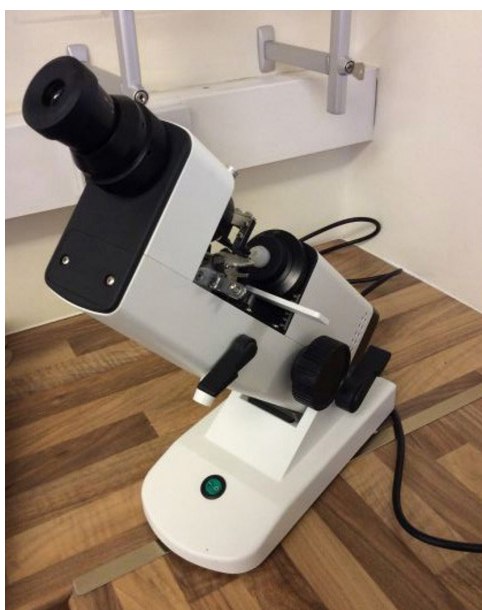
Figure 1. The focimeter used in the current study to measure a lens's back vertex dioptric power.
